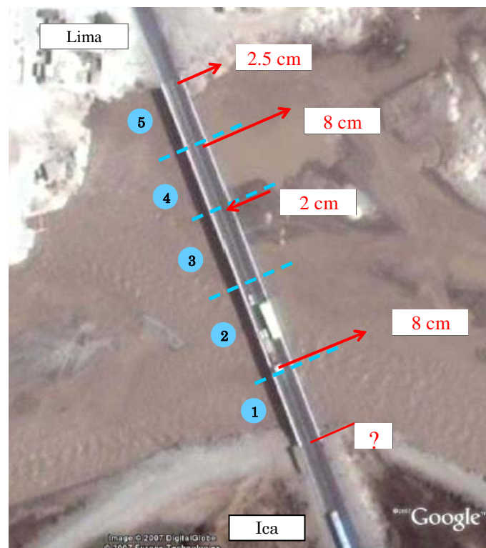
Fig. 5.24 Google earth view of the displacement of the bridge superstructure.
